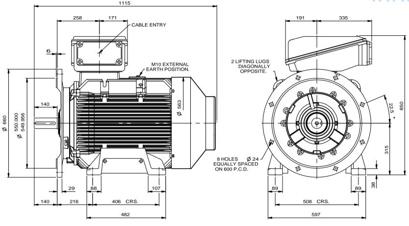
NOTE:-TERMINAL BOX CAN BE MOUNTED (LEFT OR RIGHT) BY REFITTING FEET AND LIFTING LÚGS 90° IN APPROPRIATE DIRECTIONS. CABLE ENTRY CAN BE SUPPLIED IN ANY ONE OF FOUR POSITIONS AT 90° INTERVALS.
